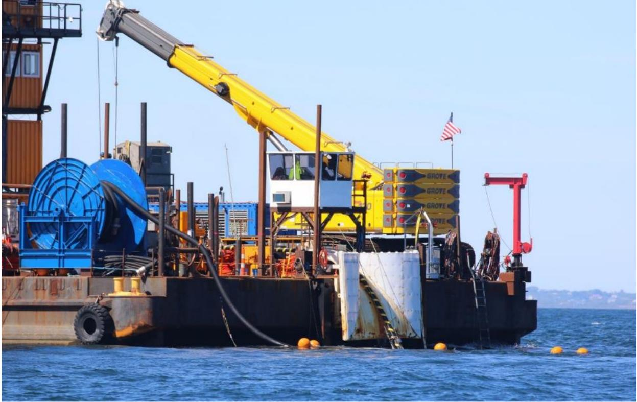
6/14/2016 Offshore – Photo 3009: BITS cable exiting chute on CLB Big Max and feed to jet plow.
