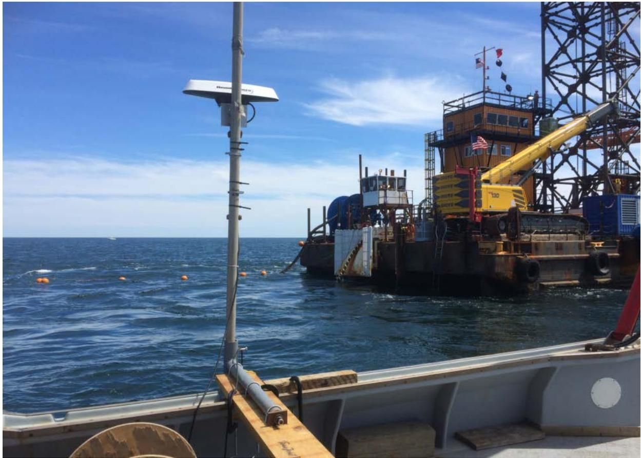
**Figure 18. ADCP and DGPS installed on a pivoting arm aboard the Jamie Hanna with the cable lay vessel Big Max and buoys marking the jet plow in the background**
