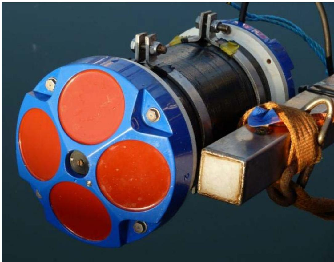
**Figure 17. RDI ADCP configured on pivoting arm**
